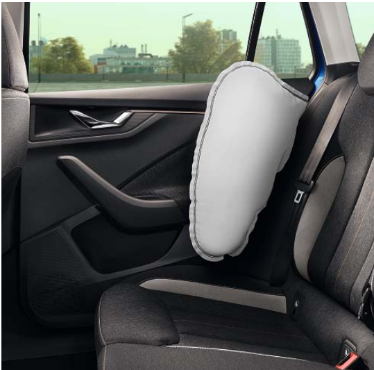
FRONT AND REAR SIDE AIRBAGS These four airbags protect the pelvis and chest of the driver and other passengers in the event of a side collision.
