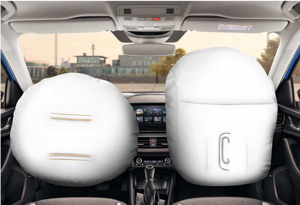
FRONT AIRBAGS While the driver airbag is enclosed in the steering wheel, the passenger airbag is located in the dashboard. If needed, this can be deactivated when a child seat is installed on the front seat.
